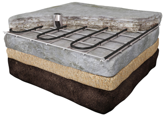
Installatie in beton
